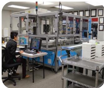
the MBV. The MBV will allow us to inspect lens powers quickly and accurately finish block lenses using the industry standard Focovision and PPOS systems. With a throughput of over 100 jobs per hour, the MBV will allow us to stay in front of lens inspection without sacrificing quality standards. This machine is something to behold.
