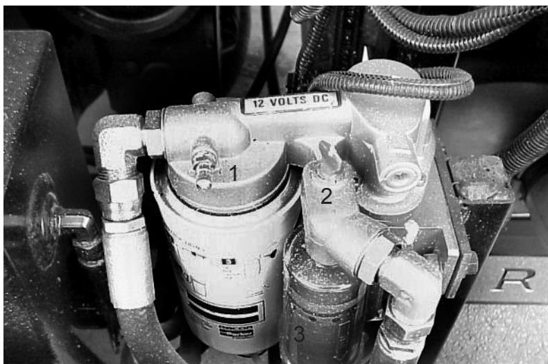
1. Schraeder valve. 2. Thumb screw. 3. Reusable filter.
