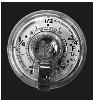
LP Tank Gauge
