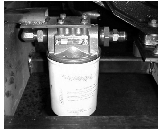
Hydraulic filter for the power steering and hydraulic cooling fans.
