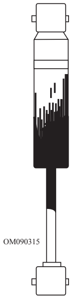
Normal shock absorber appearance after a long service period.
