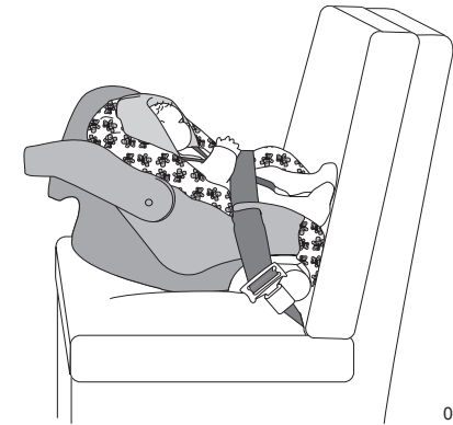
Example 1: Convertible seat facing to the rear.
