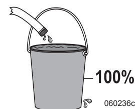
Float Charge Water (charger) slowly trickles into bucket (battery) until 100% full. Water (charger) will adjust flow to maintain level.
