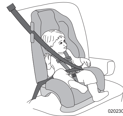
Example 2: High back booster seat facing forward.
