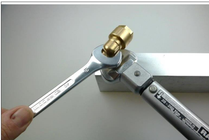
Fig. 9: Tighten the hexagonal nut using a torque wrench
