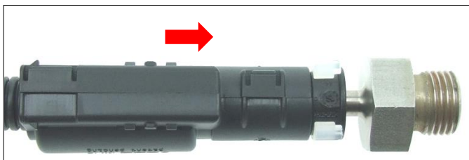
Fig. 5: Pushing the coupling as far as it will go onto the male connector; in the process the holding clip engages
