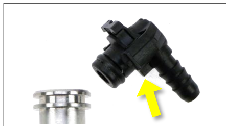
Fig. 1: Starting situation: Connector of quick connect system 246 is not assembled into the port, arms are broken
