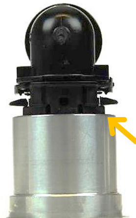
Fig. 13: Incomplete assembly plug 271
