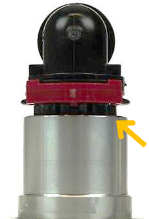
Fig. 14: Incomplete assembly plug 271 DL : blocked Double Lock
