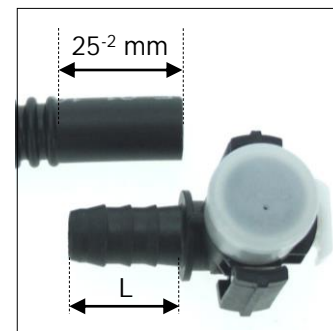
Fig. 6: Minimal length of the plain segment = length of the fir-tree
