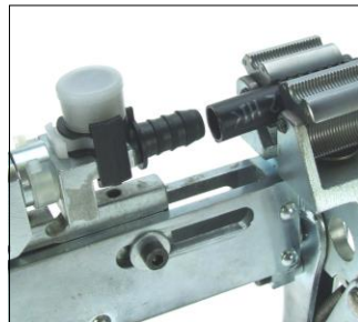
Fig. 11: Placing the tube in the jaws and the plug in the insert
